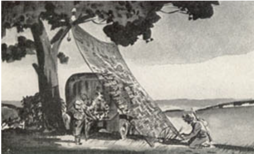
FIGURE 47 (1). An overhead screen provides good concealment. It is particularly valuable over more permanent parking places because it allows considerable freedom of movement underneath it and because vehicles can come and go while the camouflage remains in place. With this type of cover, a tight flat screen is unnecessary.
